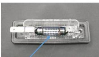
Use a TORX T20 screw drive to open two screws.
