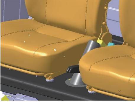
Hand brake rod is located between the two seats shown
